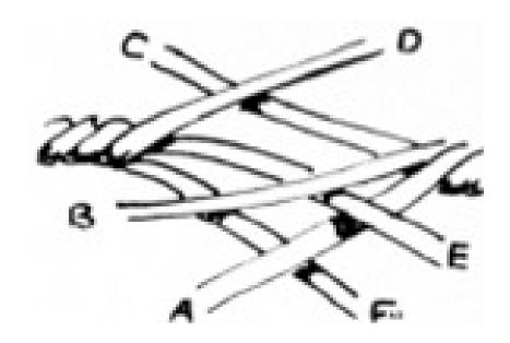
(b)Long Splicing: The strands are unlaid for a considerable length and then married as for the short splice. Then the one strand is unlaid and its married counterpart is laid along its place in the rope. The two centres are simply held with a crossover knot, and the strands thinned down and spliced as for a short splice. The end strands are finished with a crossover knot and again the strands are thinned down and finished as for a short splice.
